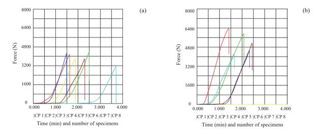
Figure 9. Normal tensile strength of glued eucalyptus laths: a) uncoated specimens; b) specimens coated on both sides with giant bamboo veneers.
