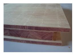
Figure 3. Experimental panels of eucalyptus laths coated with bamboo veneer (Source: Ostapiv 2011).
