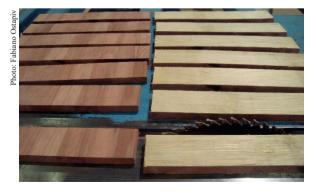
Figure 5. Specimens of *Corymbia citriodora* edge glued panel and edge glued panel reinforced with bamboo veneers.
