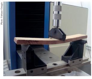
Figure 6. Bending test on bamboo battenboard specimen.
