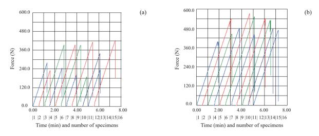
Figure 8. Normal tensile strength of eucalyptus specimens: a) uncoated; b) coated on both sides with giant bamboo veneers.
