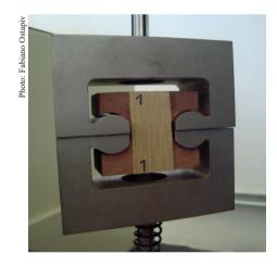
Figure 4. *Corymbia citriodora* wood specimens reinforced with giant bamboo veneers in the device and ready for testing.
