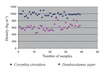
Figure 7. Density of *Corymbia citriodora* wood specimens and giant bamboo veneers.
